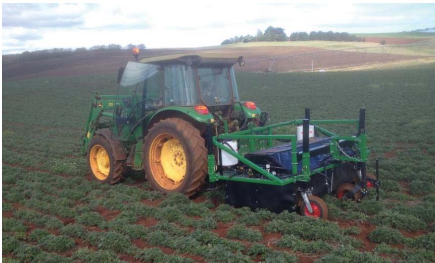
Figure 2.2 Pre-production spray rig in a field of pre-harvest seed planted pyrethrum
