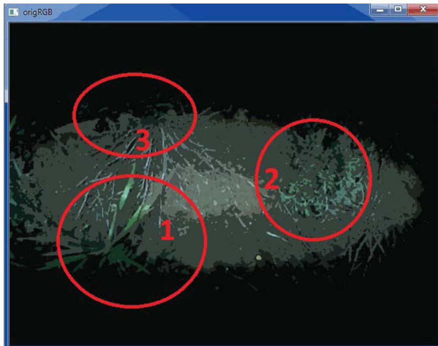
(b) Region growing segmentation technique applied to a colour image 5.1(a).
