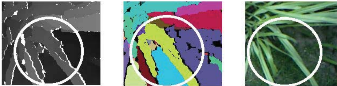
Figure 5.10: Image showing the depth image, segmented image and colour image associated with each other. The white ellipse highlights two separate leaf components that overlapped in colour and height and therefore are the one component.
