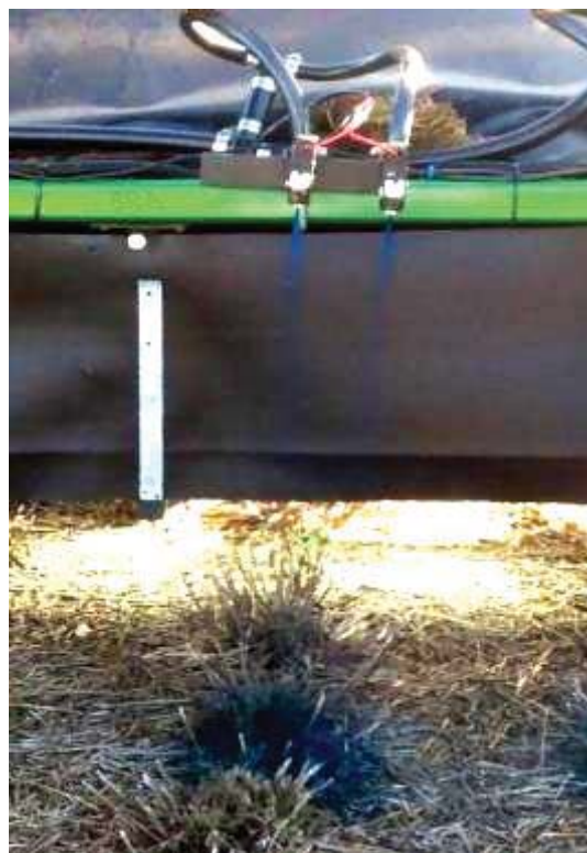
Figure 1.4: The spray system operating on-the-row
