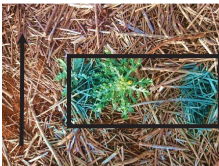
Figure 6.6: A hit with blue dye with the arrow showing the direction of the row and rectangle showing the kill zone
