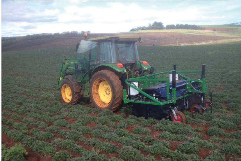
Figure 4.1: Prototype machine and Garford side-shift hitch mounted on the tractor, shown in a crop of pyrethrum.
