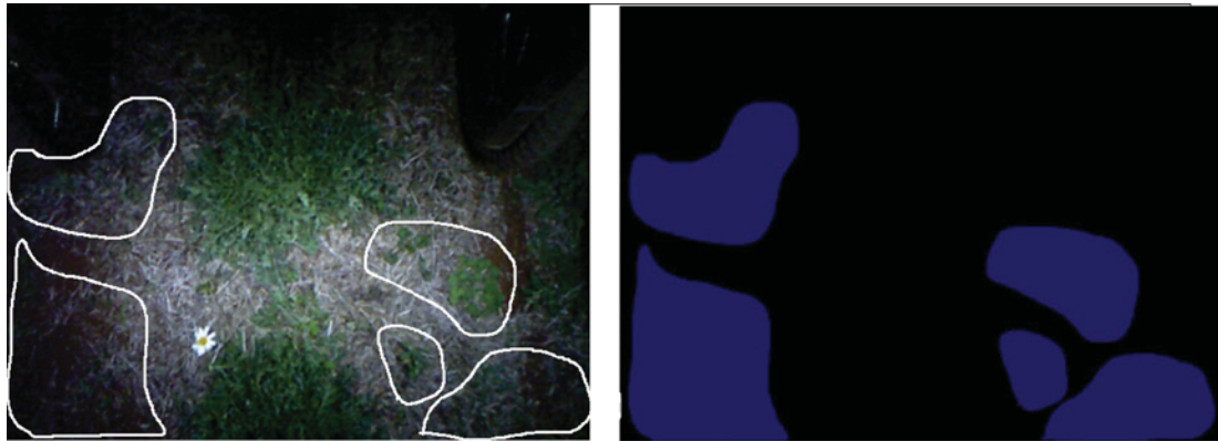
Figure 6.6: Images showing the ground truthing mask for the evaluation software. The image on the left shows the weeds circled by a mouse in white. The image on the right is the mask with the circled areas of the first image highlighted in blue.
