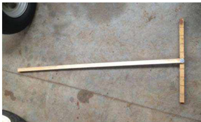
Figure 4.4 Measuring stick used for measuring accuracy of the guidance system
