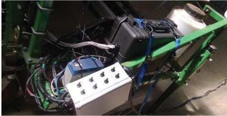
Figure 6.1: The control box ( left ) and case containing the two detect-spray computers ( right ).
