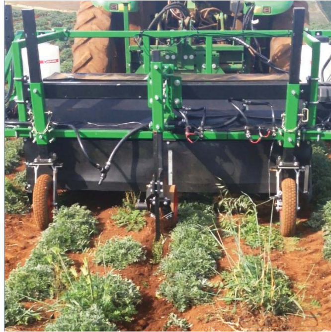
Figure 4.5: Image of the tyne assembly in operation. The coultter disk in the front of the tyne cut any vines and trash so that it could not wrap around the tyne.
