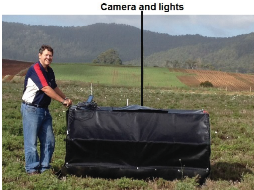
Figure 3.9: Pyrethrum data acquisition system (1 m wide \times 1.6 m long \times 1 m high) in a crop of pyrethrum March 2012. Author (1.86 m tall) to indicate scale.
