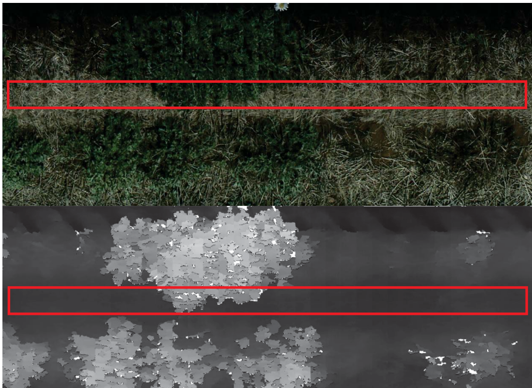
Damaged pyrethrum in the colour image and wheel track in the depth image (red rectangles)
