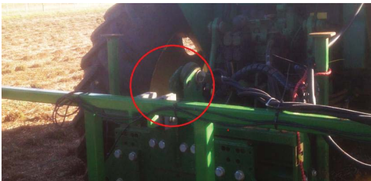
Figure 4.3: Side shift hitch in the central position
