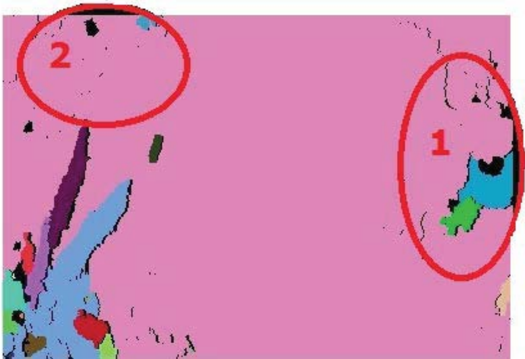
Figure 5.6: A connected components applied to the depth image associated with Figure 5.5 where each component is assigned a unique colour. Errors are apparent in red ellipse one where ground and plant merge and in red ellipse two where stubble and plant merge.
