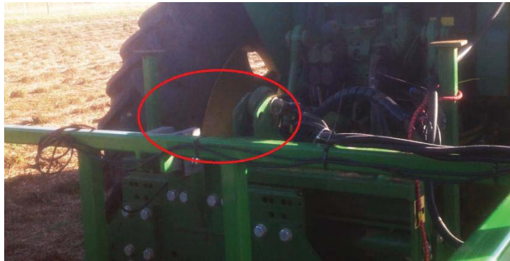
Figure 4.2: Side shift hitch in the fully left position
