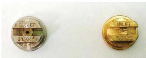
Figure 6.5: The nozzle tips used: TeeJet 1504 (left) and UniJet 150025 (right)
