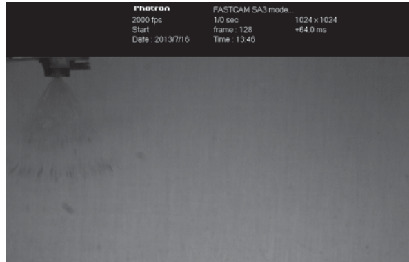
Figure 3.2: Spray pattern of an 80° nozzle after the fluid starts to flow after switch on.
