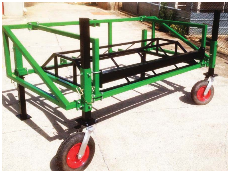
Figure 3.11: The manufactured and assembled field ready prototype frame.
