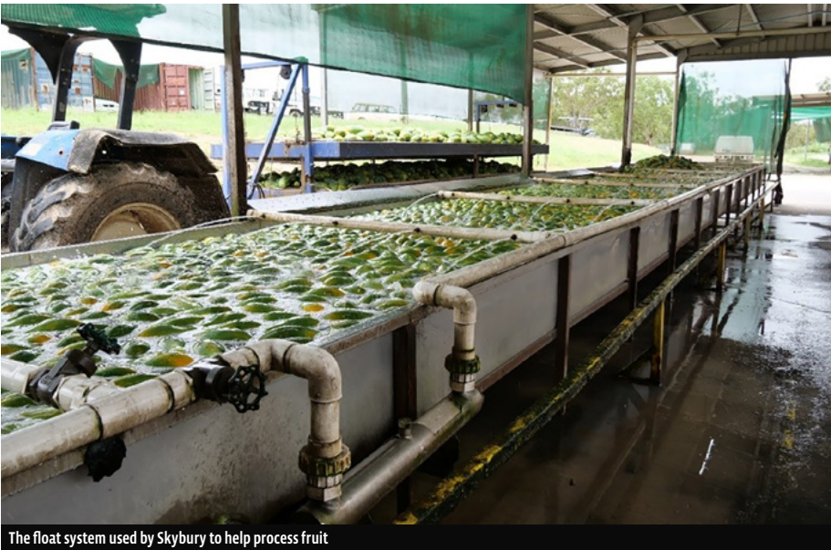
The float system used by Skybury to help process fruit
