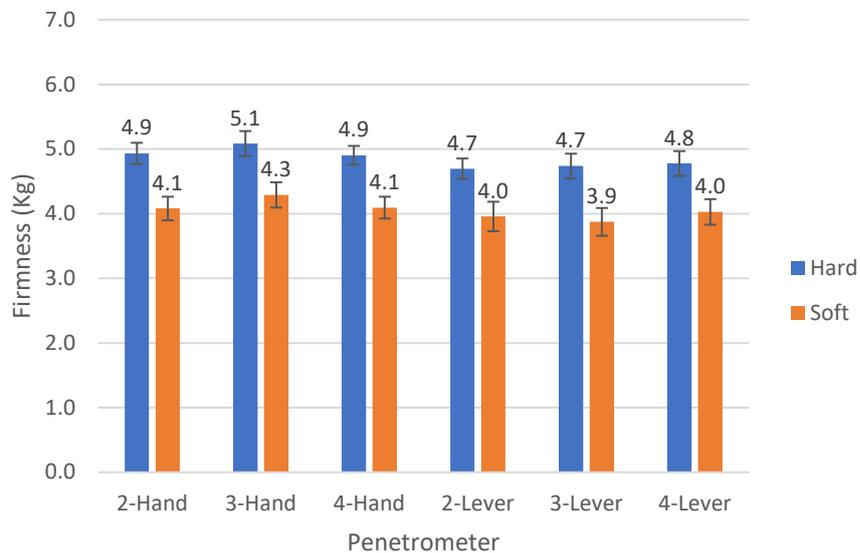
Figure 178. The firmness of oranges was measured using 3 different penetrometers of 13 kg/11 mm and a sleeve of 41.75 (protrusion 5.3).
