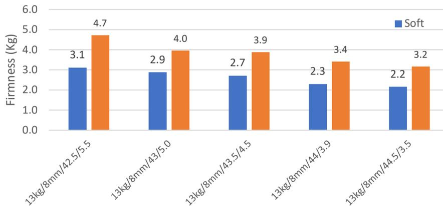
Figure 175. Firmness of oranges using 13 kg/8 mm with different sleeves.
