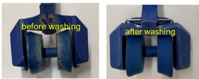
Figure 60. Effect of washing in commercial cleaners on the appearance of rollers/cups.
