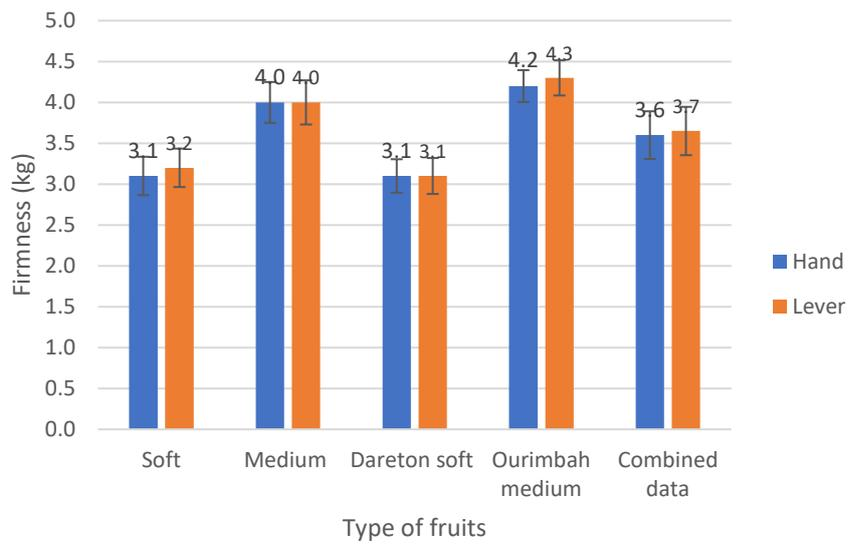
Figure 180. The firmness of oranges using different types of oranges with penetrometers of 13 kg/11 mm using the sleeve of 41.75 (protrusion 5.3)
