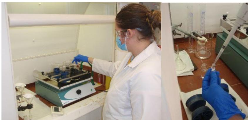
Figure 59. Washing contaminated packingline cups in solvent to assess dimethoate residues.
