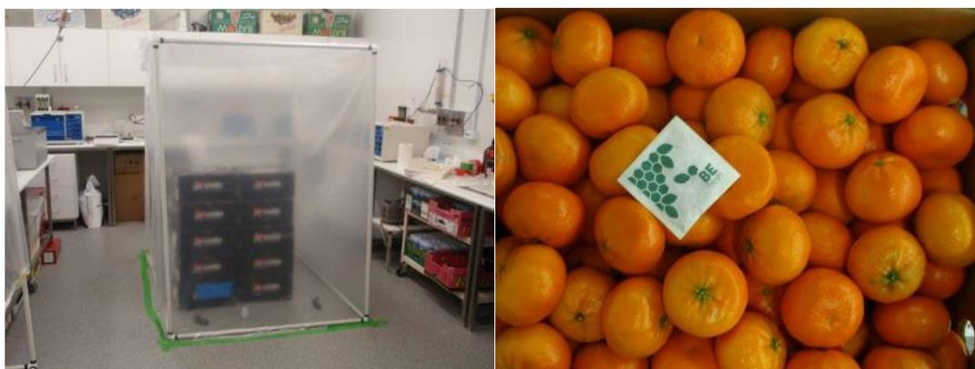
Figure 137. Treating Afourer mandarins in boxes with 1-MCP gas in a sealed tent before long-term storage (left) and with the addition of a potassium permanganate (PP) sachet within the treatment box (right).
