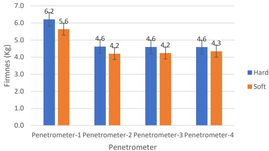
Figure 177. The firmness of oranges was measured using 4 different penetrometers of 143 kg/11 mm and a sleeve of 41.75 (protrusion 5.3).
