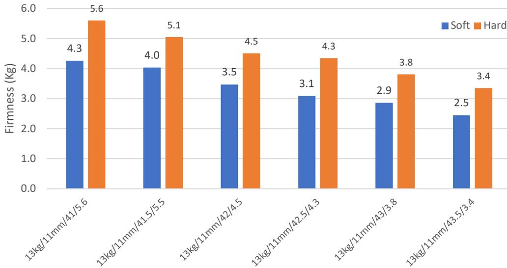
Figure 174. Firmness of Navel oranges using 13 kg/11 mm with different sleeves.
