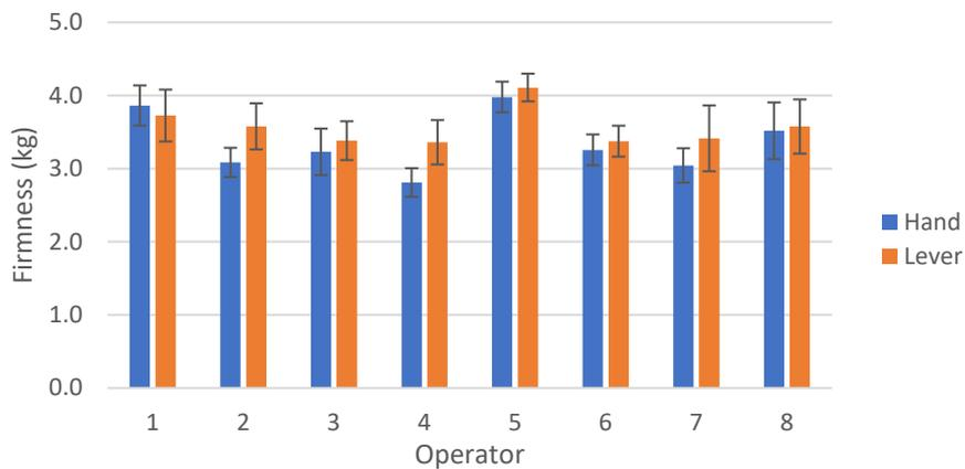
Figure 181. Firmness of oranges by different operators using penetrometers of 13 kg/11 mm with sleeve size of 41.75 (protrusion 5.3)
