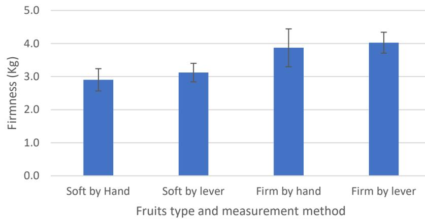
Figure 182. Firmness of oranges was assessed by band and lever for soft and firm oranges using penetrometers of 13 kg/11 mm with sleeve size of 41.75 (protrusion 5.3)
