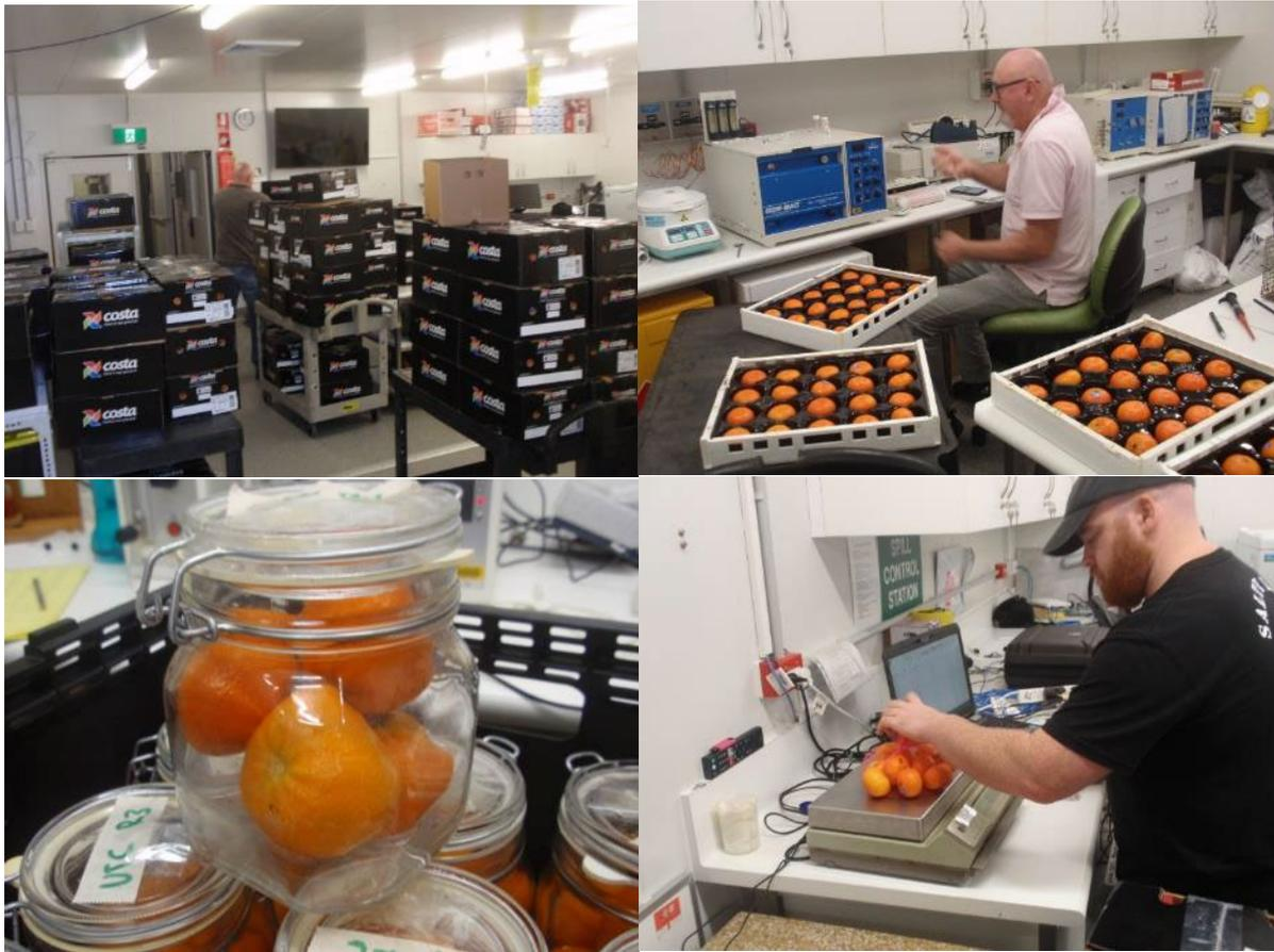
Figure 138. Setting up the storage trial and measuring fruit quality (ethylene, respiration rate and weight loss) during storage at NSW Department of Primary Industries.
