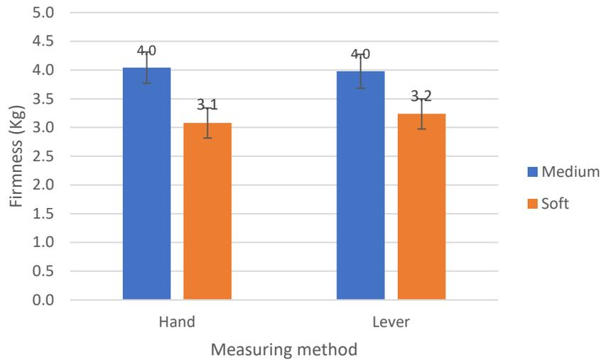
Figure 179. Firmness of oranges (soft and medium) using penetrometers of 13 kg/11 mm with sleeve of 41.75 (protrusion 5.3)
