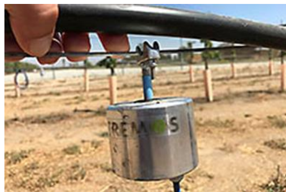
A custom made, prototype vibration emitter is placed on a trellis during field trials at the Crop Diseases, Pests and Genetics Research Unit in Parlier California. Rodrigo Krugner (D4202-1)
