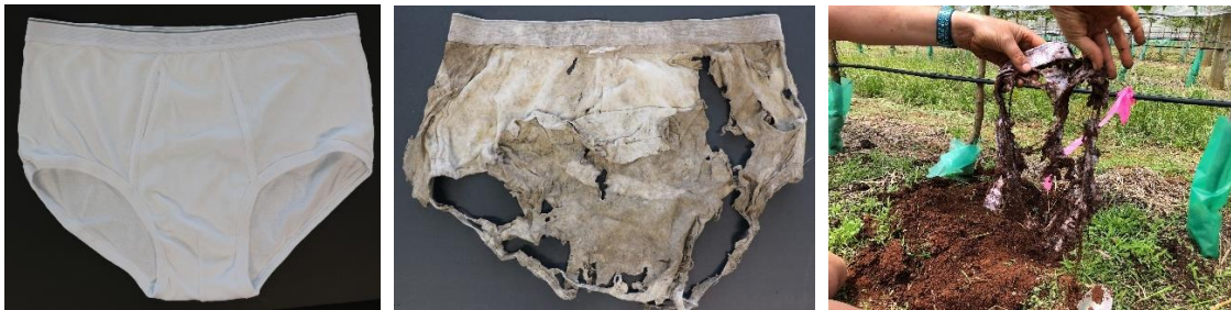
Figure 8: Cotton undies for checking soil biological activity. Note lack of degradation of synthetic elastic and thread in photo on right.
