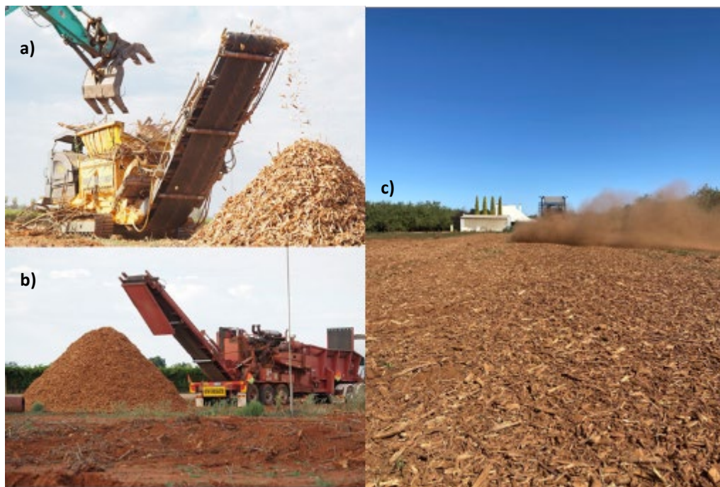
Figure 1. Tree chipping with a) Tana Shark Waste Shredder, b) Morbark Wood Hog, and spreading with c) Penta Manure Spreader. Photos D. Jaensch, Almond Board of Australia.
