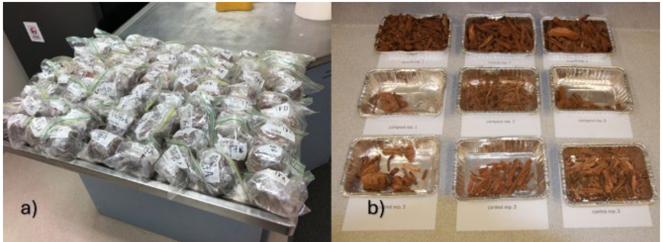
Figure 6. Laboratory analysis of a) undisturbed soil cores and b) wood chip content of soil.
