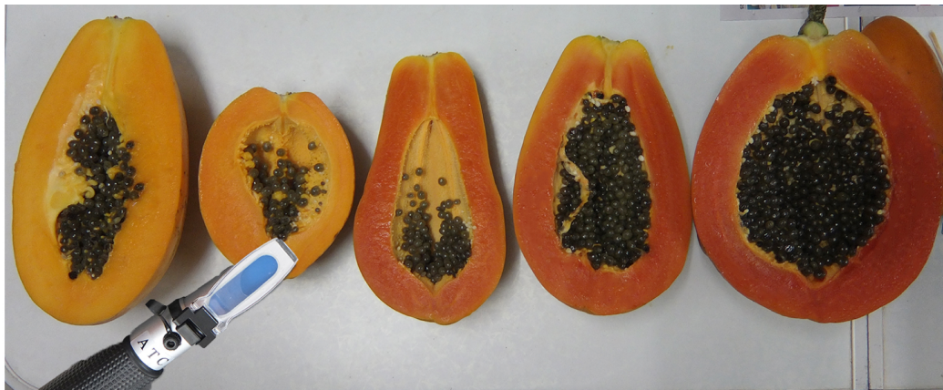
Figure 28: Measurement for flesh sweetness using a hand held refractometer
