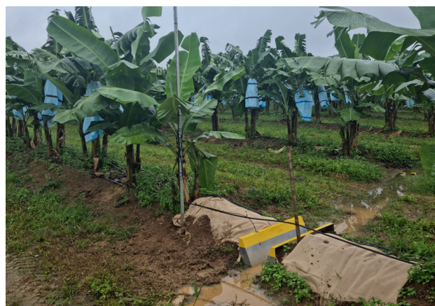
Runoff flume with flow rate monitoring
